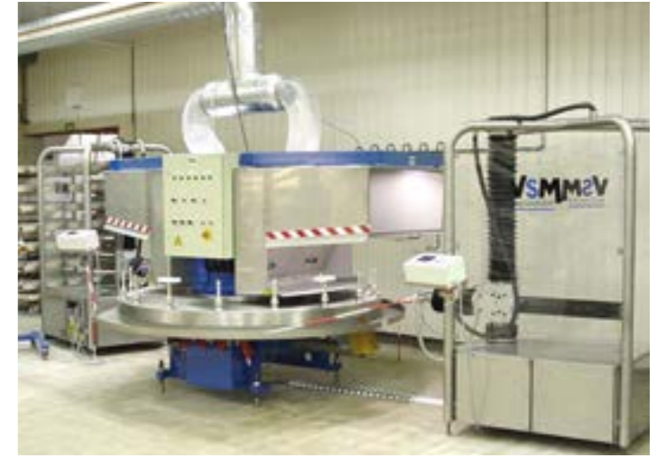
M-CAF-2-D-16-K 2 Coat-A-Flex, 16 spindles. For two colour application, by turning over the products.
