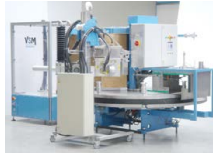
M-CAF-1-B-8-D-CB 1 robot, 8 spindles With a closed spindle cleaning booth and dryer.
