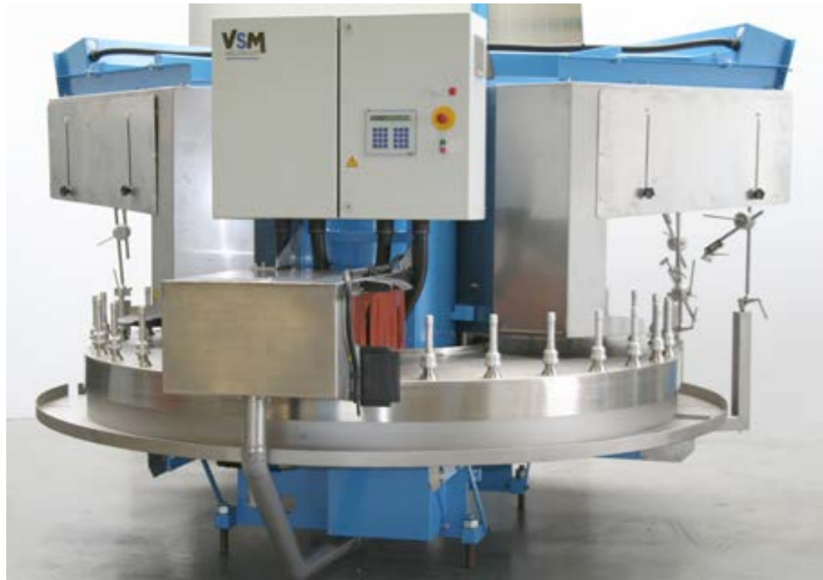
M-D-2-6-32-CB 2 spray booths, 6 spray positions, 32 spindles With an open spindle cleaning booth.
