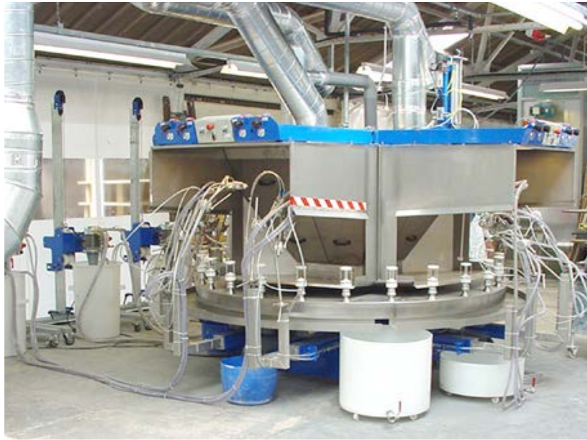
M-D-3-9-24 3 spray booths, 9 spray positions, 24 spindles.
