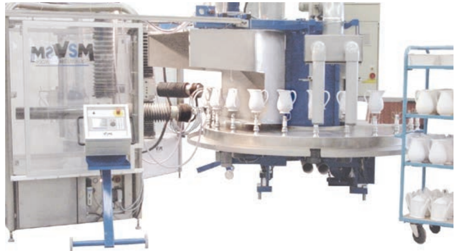
M-CAF-1-B-8-D-CB 1 robot, 8 spindles With a closed spindle cleaning booth and dryer.
