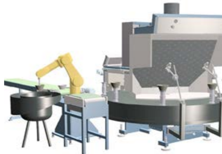
M-C-8-DR 1 spray booth, 2 spray positions, 8 spindles With a dipping robot.
